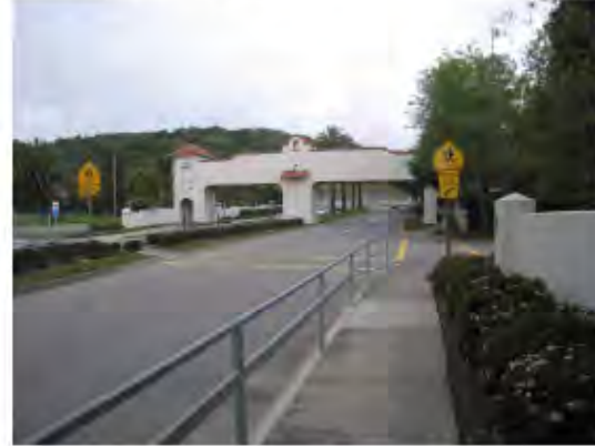
Facing west on Main Gate Road Existing crosswalk signs should be replaced by new, lower FYG signs
